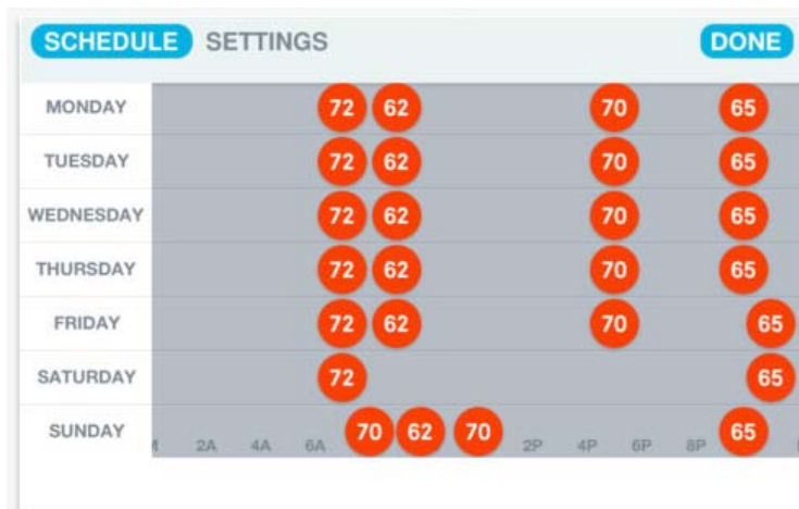
Figure 2: A screenshot of the iPhone GUI for programming the Nest Thermostat illustrates how Internet-connected applications can improve the user experience of core device functions.
